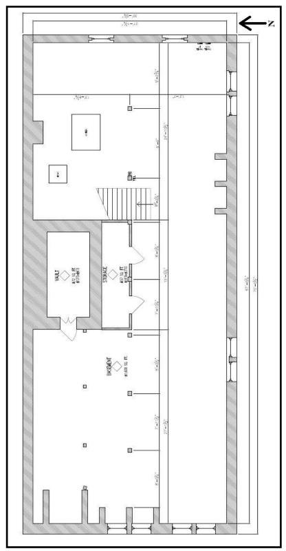
The basement floors are concrete with a dirt floor at the southwest corner; walls are concrete; and ceilings are open wood framing with wood support columns. It is partitioned to a storage closet and a walk-in vault room, with remainder of the basement open. The basement contains HVAC for the building and is used only as storage.
