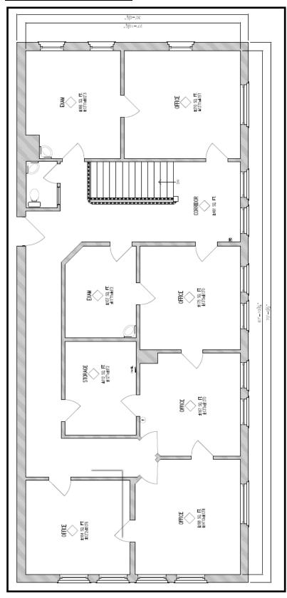
At this time, the second level is vacant. Currently, the floors are wood plank; walls are plaster; and the high ceilings are plaster. There are windows along the west, south, and east sides of the second level that are woodframed and single pane. Access between rooms is provided from doorways with transom windows above the doors.
