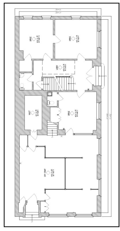
The main level is partitioned to the front lobby area, a vault room, two restrooms, and three offices. The front lobby area contains half walls that are masonry constructed from its original use as a bank. One office is centrally located along the south wall and the other two offices are located along the east wall.
